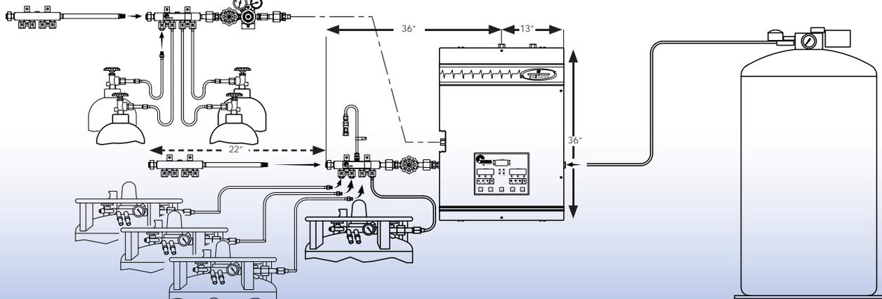
Microbulk primary x Cryogenic liquid cylinder secondary
